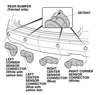
12. Install the right corner sensor clip (black), the left corner sensor clip (white), the right center sensor clip (black), and the left center sensor clip (white).
