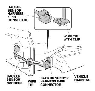
35. Secure the backup sensor harness to the vehicle harness using a wire tie.
