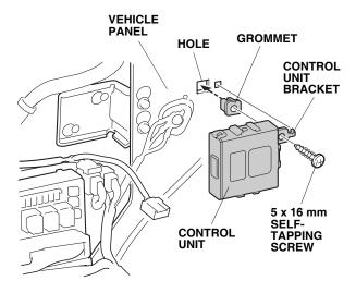
41. Position the control unit bracket on the grommet, and install the 5 x 16 mm self-tapping screw.
