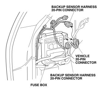
Clean the fuse case with isopropyl alcohol. Attach the fuse label (BACKUP SENSOR 2A) to the fuse case.
