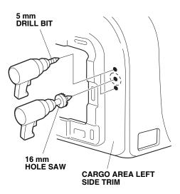
48. Route the buzzer harness through the 16 mm hole. With the buzzer switch facing up, install the buzzer with two 4 x 14 mm self-tapping screws with two washers.
