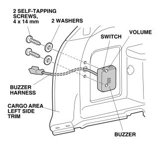
49. Plug the buzzer harness 2-pin connector into the backup sensor harness 2-pin connector. Secure the buzzer harness 2-pin connector to the vehicle harness using one wire tie.
