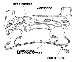
14. Secure the seven subharness clips to the seven rear bumper tabs.
