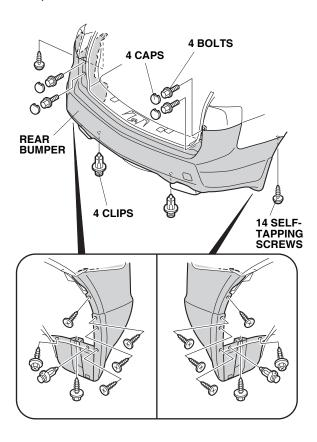
4. With the help of an assistant, remove the rear bumper (four hooks). Place the rear bumper on a blanket to prevent damage.
