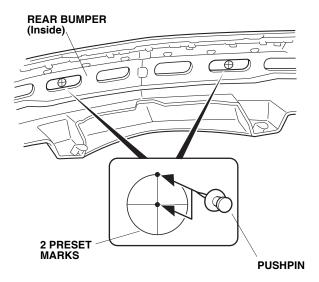
6. Working from the outside (painted side) of the bumper, use a 3 mm drill bit to drill four holes in the rear bumper at the pierced holes you made in step 5. Wear eye protection.
