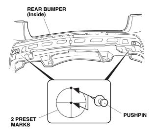
9. Working from the outside (painted side) of the bumper, use a 3 mm drill bit to drill four holes in the rear bumper at the pierced holes you made in step 6. Wear eye protection.
