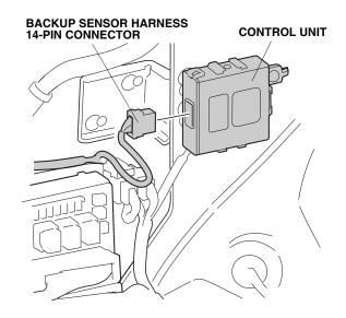
43. Secure the backup sensor harness to the vehicle harness using four wire ties.
