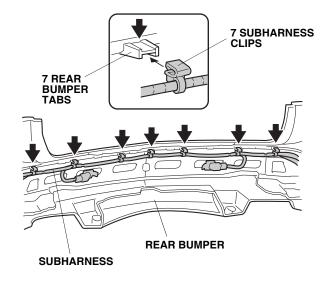
15. Secure the two subharness clips to the left and right corner sensor clips.
