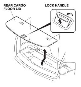
17. Turn the knobs, then remove the cover from the rear cargo tray.
