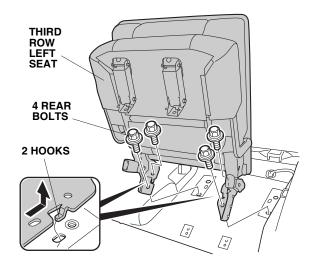
24. Release the two hooks by moving the third row left seat rearward, then remove the third row left seat.
