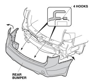
5. On the inside of the rear bumper, locate the two preset marks. Using a pushpin, pierce through the rear bumper at the four locations shown.
