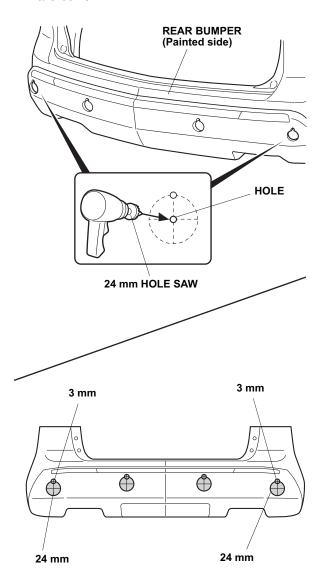
11. Install the center sensors and corner sensors into the rear bumper.
