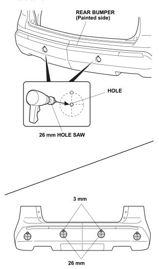
8. On the inside of the rear bumper, locate the two preset marks. Using a pushpin, pierce through the rear bumper at the four locations shown.
