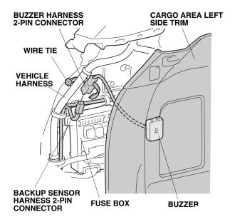
50. Plug in the vehicle connector unplugged in step 29, then reinstall the cargo area left side trim, two lower tie-down hooks, two lower clips, and screw. Check that all clips and retaining tabs are installed securely.
