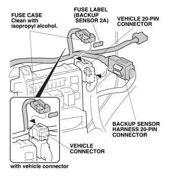
38. Clip the fuse case and backup sensor harness 20-pin connector to the vehicle 20-pin connector.
