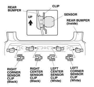
13. Route the subharness along the rear bumper. Plug the subharness 2-pin connectors into the sensors.
